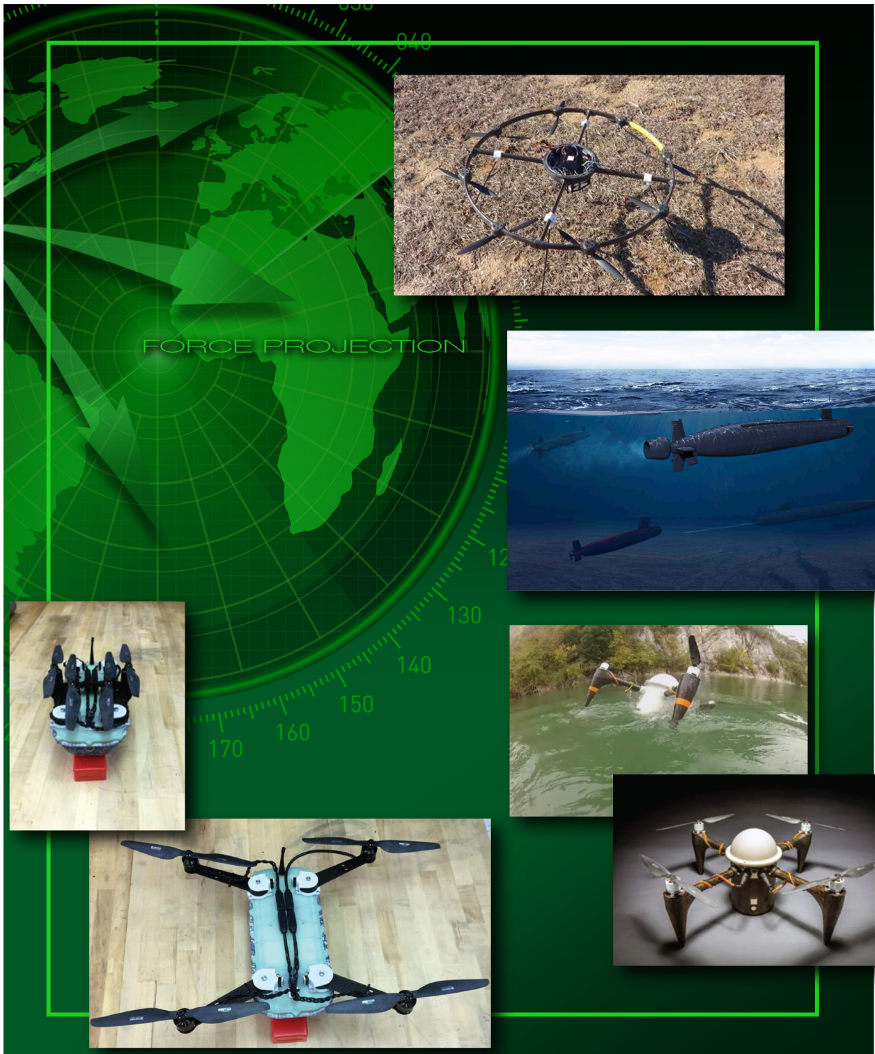
Examples of transformational capabilities delivered to the warfighter. Images, clockwise from top: an airframe constructed using novel additive manufacturing techniques; technologies extending the reach and influence of U.S. submarines in naval warfare; the Corrosion Resistant Aerial Covert Unmanned Nautical System (CRACUNS); and the Mini-CRACUNS platform model showing folding arms for stowage inside an unmanned underwater vehicle.
