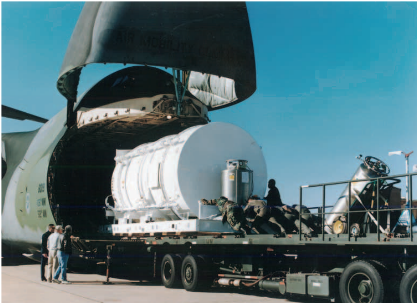
Figure 6. MSX shipping container, with the spacecraft inside, being loaded into the C-5 for flight to Vandenberg Air Force Base. The dewar at the end of the transporter cart supplies the nitrogen for the instrument purge during transport; the line is visible along the near side of the container. The dewar to the far right supplies the SPIRIT III door dewar with argon if required.
